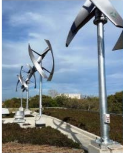
Figure 1.4 Darrieus-Type Wind Turbine. Retrieved from https://images.nrel.gov/bp/#/folder/207425/51085242 'NREL Image Gallery', Image number: 42794.jpg. Reprinted with permission.
